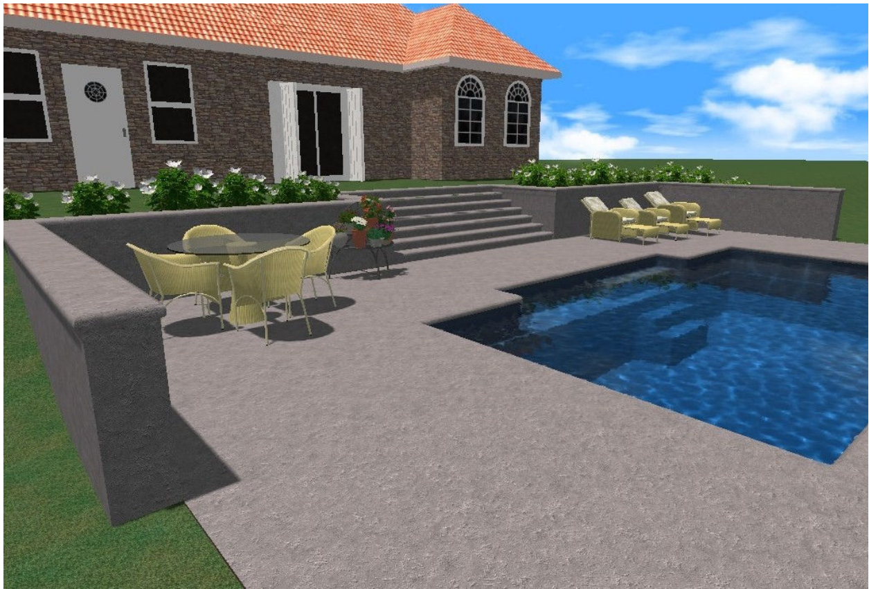
Poured concrete wall with recessed concrete steps
